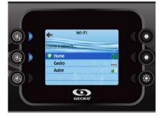
If no password is required the in.touch will connect automatically.
