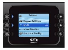
For the Wi-Fi menu to appear in the Settings menu your in.touch module must be equipped with software version 11.00 or higher. This menu allows you to connect your in.touch module to a Wi-Fi network or to change its network.
